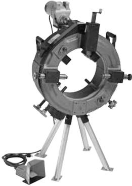
Includes riser blocks and grooving heads for cut grooving 4 – 12" ductile iron rigid groove. Power drive supplied requires 120 volt, 11.5 amp electrical supply. Stand included at no extra charge.
