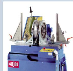
4001 Heating Element Butt Welding Shop Machine
